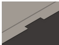
Figure 7. Cut out in the rear wall of the drawer tray
